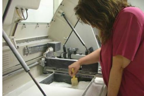
A Veterans Workshop participant carefully removes her designed and printed part from the build box on a Z-Corp 510 additive manufacturing printer.
